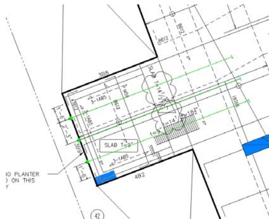
Figure 9: Cantilevered balcony utilizing post-tensioning
